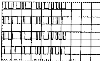
TOP IC101 pin 30 (DATA) MIDDLE IC101 pin 31 (CLK) BOTTOM IC101 pin 22 (LATCH) 5V/DIV. TB 50µSEC/DIV.
